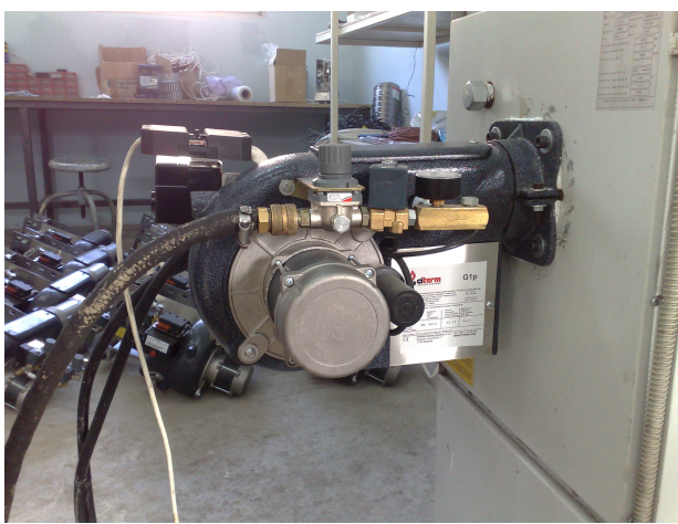
Picture 3. Burner type G1P, manufacturer „CITERM HEATING SYSTEMS“
